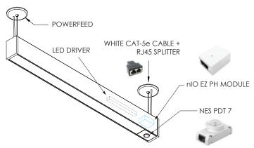
ALW will provide a CAT5e cable and RJ45 splitter for nLight Wired specs
